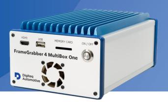
FrameGrabber 4 MultiBox One is part of Digiteq Automotive FrameGrabber 4 (FG4) modular ecosystem. It is a powerful, standalone and versatile solution not only for video applications. It is the best choice for laboratory and in-car applications thanks to its compact dimensions.
