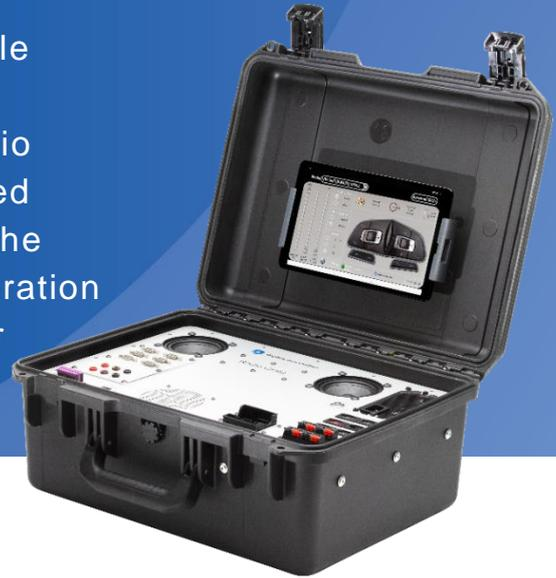
Part of the presentation stand is a tablet with the Android operating system. The tablet is connected to the stand via Wi-Fi and is used to control the built-in computer equipped with simulations of the car environment. At the same time, it is used to control the switching of artificial loads intended for speaker outputs or to bridge an audio signal output to external terminals.
